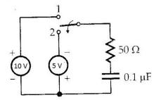
In the circuit shown in figure.(11) the switch S is in position 1 and the circuit (10) attained its steady state. The switch S is transferred to position 2 at time t=0.
