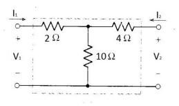
6 Check for symmetry and reciprocity of a two port network in z parameter (5) representation shown in figure
